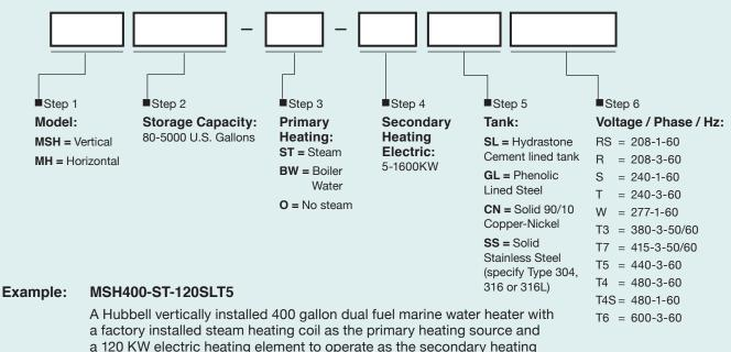
a factory installed steam heating coll as the primary heating source and a 120 KW electric heating element to operate as the secondary heating source. Tank is cement lined. Power required is 440 VAC, 3 phase, 60 Hz. Please note that steam heating capacity and construction features are not identified in the model number and therefore must be noted in the written specifications.
